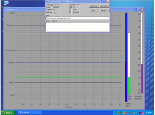
above the 'optimal temperature' line called 'high temp. warning', 'experiment stop', and 'warm up'.
